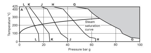
The product **must not** be used in this region or beyond the parameter of the PMA or TMA of the relative end connection.
